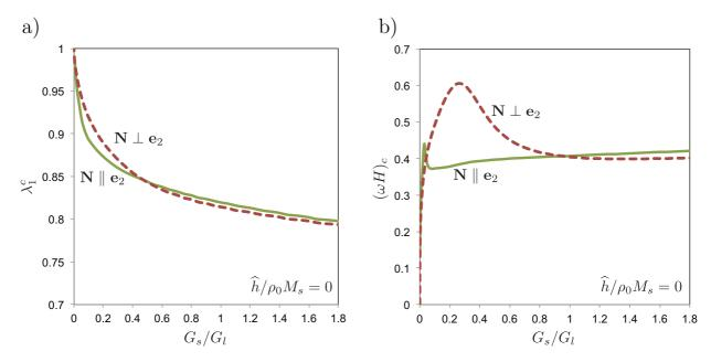
Figure 3: Critical values of (a) the interface stretch ratio  $\lambda_1^c$  and (b) the corresponding wavenumber  $(\omega H)_c$  as functions of the substrate-layer shear moduli ratio  $G_s/G_l$ , in the absence of external magnetic field  $(\hat{h}/\rho_0 M_s = 0)$ . The particle chains are either parallel ( $\mathbf{N} \parallel \mathbf{e}_2$  – solid line) or perpendicular ( $\mathbf{N} \perp \mathbf{e}_2$  – dashed line) to the thickness direction  $\mathbf{e}_2$ .
