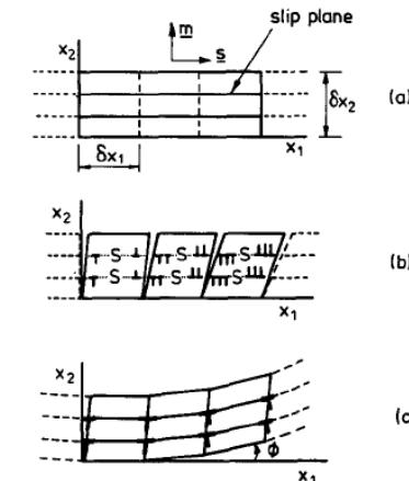
Fig. 4. Sketch showing that a gradient of slip in the  $x_1$  direction causes a density  $\rho_G$  of geometrically necessary dislocations to be stored. Plastic slip is assumed to occur on a single slip system with unit normal  $\mathbf{m}$  aligned with the  $x_2$  axis, and slip direction  $\mathbf{s}$  aligned with the  $x_1$  axis.
