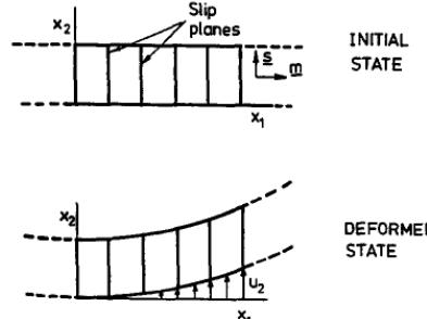
Fig. 3. A beam subjected to non-uniform shear. Plastic slip is assumed to occur on a single slip system with unit normal  $\mathbf{m}$  aligned with the  $x_1$  axis, and slip direction  $\mathbf{s}$  aligned with the  $x_2$  axis.
